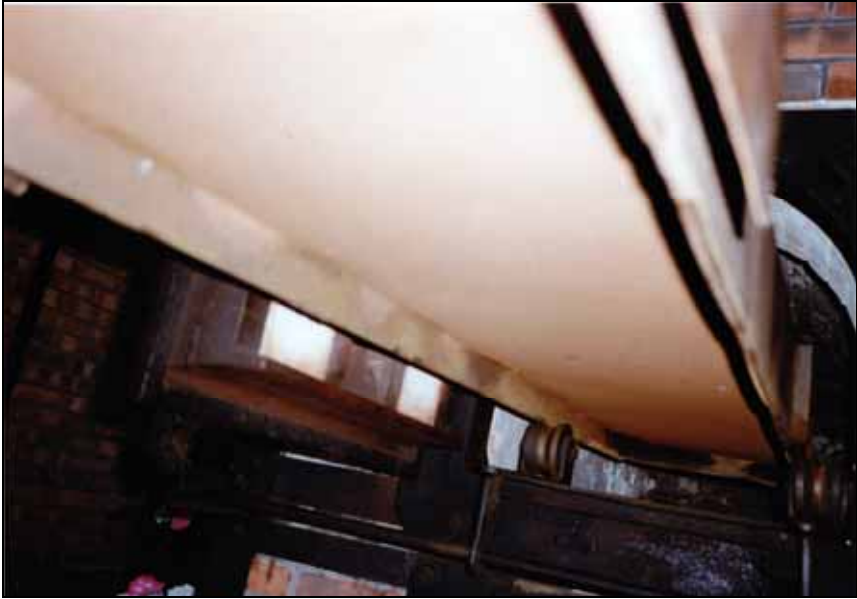
Document 42: Crematorium of Buchenwald. Topf triple-muffle coke-fired oven. Central muffle. Corpse introduction cart. Lower side. Rims of the stretcher running on the rollers. © Carlo Mattogno.
